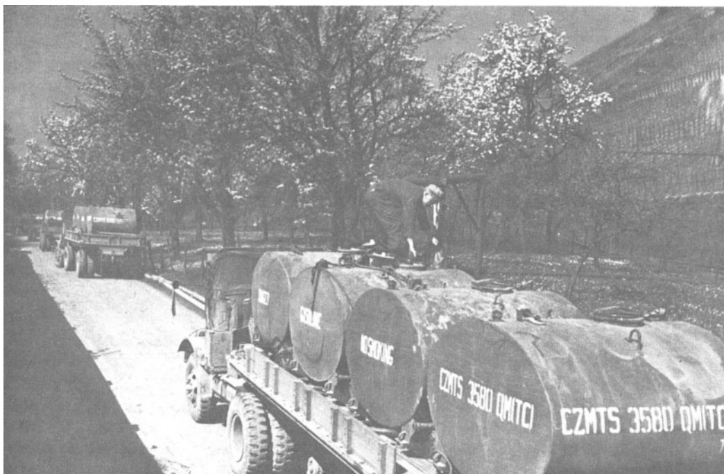
FOUR 750-GALLON SKID TANKS mounted on 10-ton semitrailers used for transporting gasoline in bulk.
